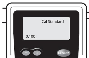
Use the **+ or -** button to change the number to the BAC level of standard you will be calibrating to. It should be the same as on the bottle of certified solution or as your altitude corrected standard, if using a dry gas tank. (See p. 14)
