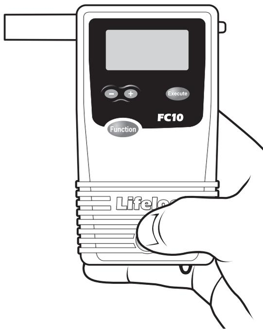
Press and hold the Power button on the bottom of the front of the unit until it beeps. The FC10 performs an automatic internal diagnostics check.
