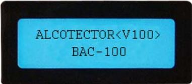
1. Press "On/Off" button to turn on the Alcotector. Software vision and model number displayed on screen.
